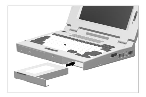
Figure 5-6. Using the Battery Pack as a Counterweight
